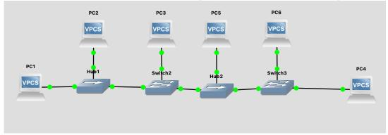
**Solution:** The request is seen by every PC in the network, because a request is send to the broadcast address. The reply will be seen on PC1 as the receiver of the response, and PC2, because the packet is forwarded to all clients connected to hub1.
