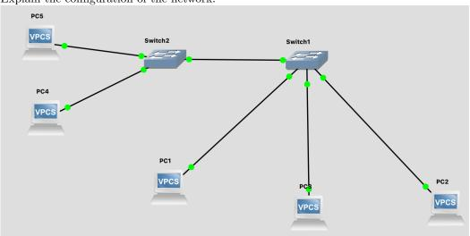
**Solution:** PC2 and PC4 are in a different VLAN than PC1, 3 and 5. The link between the switches is configured as a VLAN-trunk.
