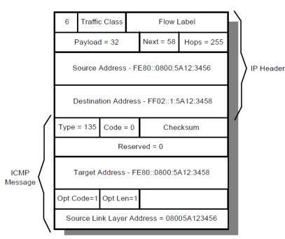
The IPv6 Destination Address is the **solicited node address** for the target workstation (a special type of **multicast**). Every workstation must respond to its own solicited node address but other workstations ignore it.
