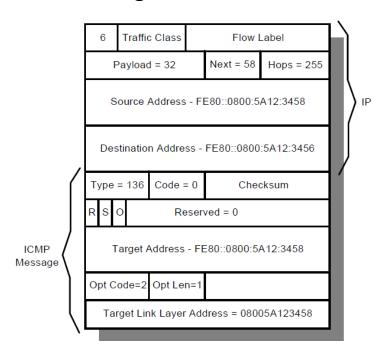
The neighbor advertisement is addressed directly back to workstation A. The ICMP message option contains the target IP address together with the target's link layer (MAC) address.
