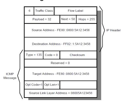
**Target address** is the known IP address of the target workstation.
