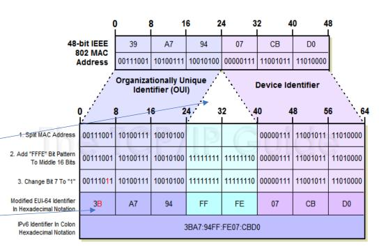
64-Bit IPv6 Modified EUI-64 Interface Identifier
