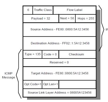
The Ethernet Source Address (LLA) is useful to the target workstation and saves it from having to initiate a neighbor discovery process of its own when it sends a packet back to the source workstation.
