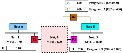
Host B is connected to the network via two different paths. Now it can happen that e.B. the first two fragments come via R3, but the last one via R2. None of the routers involved "sees" all fragments, the reassembly is only possible at the destination,
