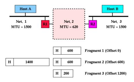
Host A sends an IP datagram with a payload size of 1400 bytes. Router 1 breaks down the datagram into 3 fragments. Host B reassembles the 3 fragments like the.
